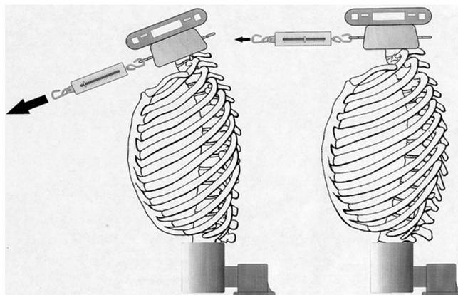
Figure 1. A cadaveric torso is shown clamped in the erect posture. A digital goniometer was attached to the upper end cap. In this left lateral view the torso is being flexed under the application of the 25-N force applied manually through a spring balance.
